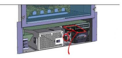
Lift the flap and disconnect the quick connection
